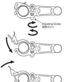
Prior to installing SGL-300S, turn the Adjusting Screw to roughly adjust the clamp opening size. On this M-size Space-Mount clamp, the fully screwed position will fit 22mm, and the fully loosened position will fit 29mm diameter.
