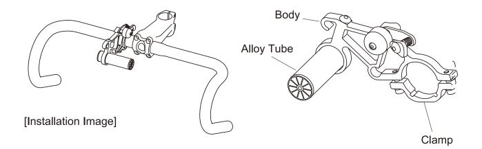
If your handlebar is 22mm (7/8") diameter, insert the plastic shim into the clamp.
