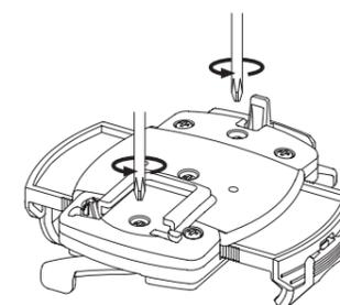
The center chrome plated screw holds the arm. Loosen it to adjust the arm position.
