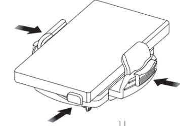
Place the phone and shut the wings to hold the phone temporarily.
