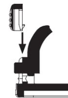
While pushing the hook fully toward the wing end, slide down the shim to the pins to fix. Make sure you fully push down the shim.
