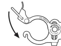
Wrap the protection tape around the handlebar. Put the clamp on it and shut the arm. Hook the metal ring.
