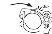
If you hear clicking sound when completely closing the lever, it's the sign of correct installation. If you don't hear any sound, the clamp is still loose. Release the lever and tighten the adjusting screw a little more.
