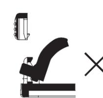
If the hook has been slanted, the shim cannot be installed.
