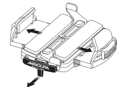
**Re-pushing the wings after clamping the phone could release the lock automatically. Make sure the red lock lever is fully engaged before riding.**
