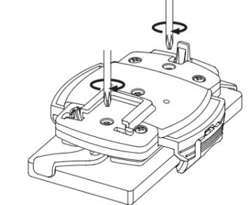
Slide both arms until they touch the phone case. Tighten the screw to fix the position.
