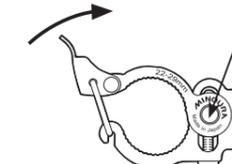
Adjust the side screw to be as you feel some resistance when the lever comes to the mid point on its stroke.
