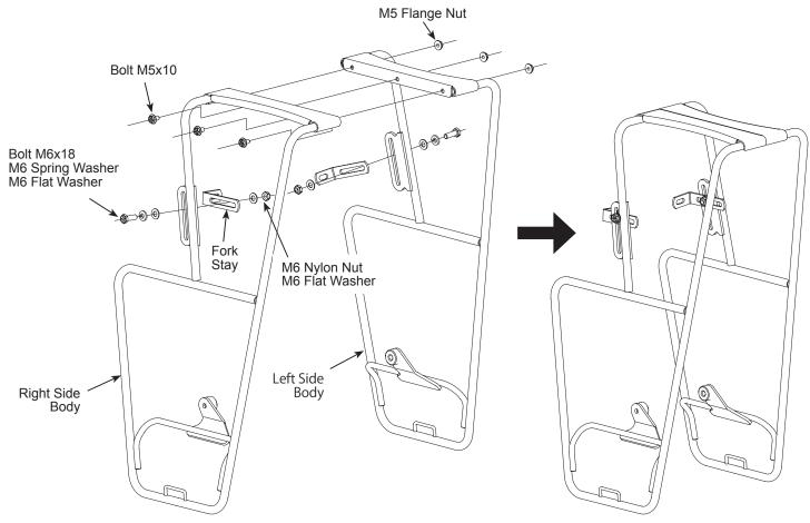
The mounting band should be installed at the point approximately 250mm above from the front wheel axle. Wind the plastic shim (protector) around the stanchon tube and put the metal band on it. (The following images show the bracket direction for the right side fork.)
