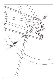
Install on the outside of the leftside chain-stay with the quick release skewer for the rear wheel.
