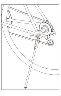
The kickstand will be locked by tightening the quick release skewer.
