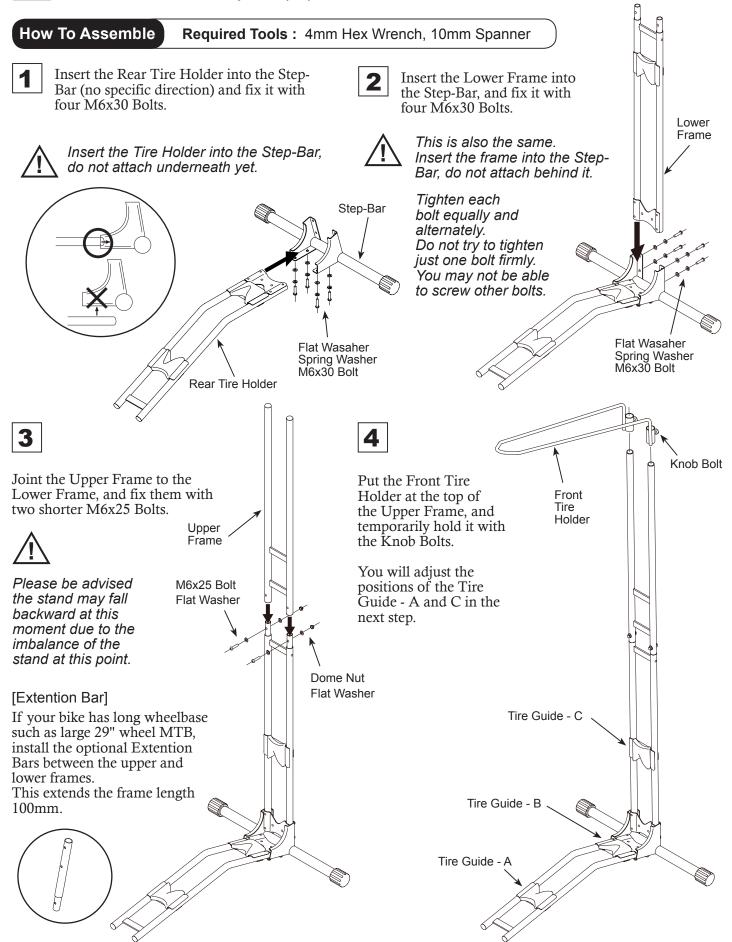
Adjust the positions of the Tire Guide - A and C precisely to fit to your exact tire size.
