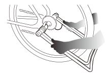
Hold the DS-30MP with both hands, and hook the left side coupling (the larger one) onto the left side rear wheel hub end (the lever side on Q/R).
