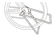
Open the legs and stand the bike. Depending on the Q/R lever design, hold the lever from top and bottom side by rotating the coupling inner holder. (refer to the bottom of the page)
