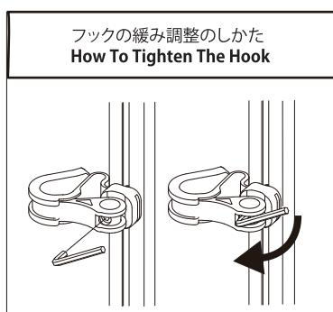
If the hook has been loosened accidentally, raise up the hook and slightly tighten the inside bolt with 4mm hex wrench.
