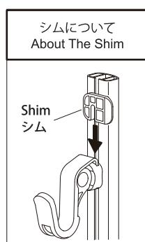
If the bike is not fully vertical, try inserting the shim between either the top or bottom hook and the pillar.
