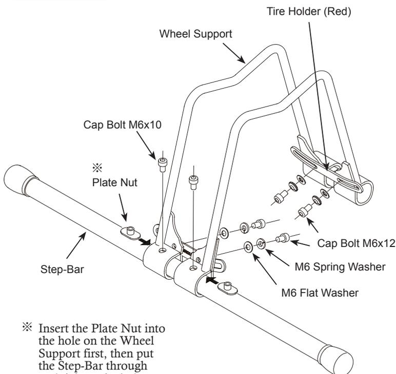
※ Insert the Plate Nut into the hole on the Wheel Support first, then put the Step-Bar through and tighten the bolt from outside to hold.
