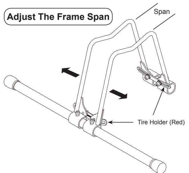
Adjust the Wheel Support frame span to fit the actual tire width.
