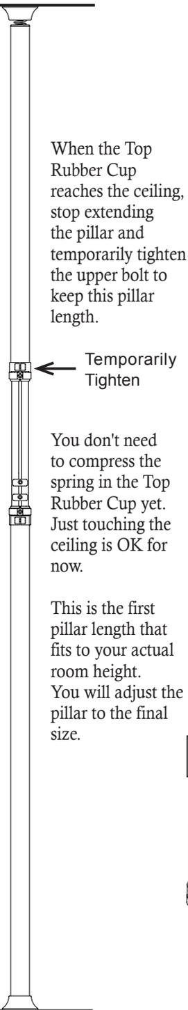
When the Top Rubber Cup reaches the ceiling, stop extending the pillar and temporarily tighten the upper bolt to keep this pillar length.
