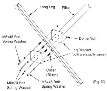
Use the longer M6x70 Bolts to the center 2 holes for screwing into the Pillar.
