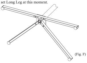
Put the longer M6x70 Bolt to the end hole on the Short Leg, then screw it into the Pillar.
