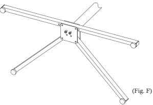
Put the longer M6x70 Bolt to the end hole on the Short Leg, then screw it into the Pillar.
