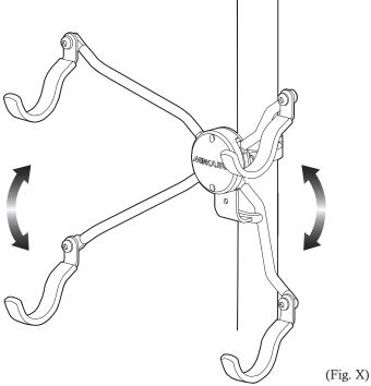
To change the arm angle, loosen the Arm Connecting Bolt through the center hole first, loosen the backside Arm Angle Fixing Bolt on each arm, then change the arm angle by hand.
