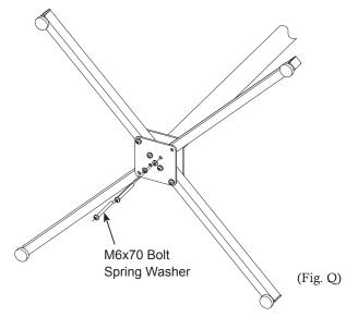
Put the shorter M6x45 Bolt to other hole, sandlwich the Short Leg with two Leg Brackets, then screw to the Dome Nut.
