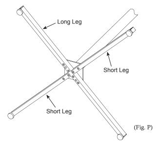
Put the longer M6x70 Bolt to the end hole on the Short Leg, then screw into the Pillar.
