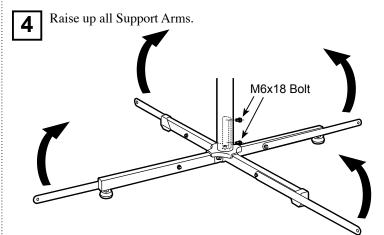
Assemble a pair of Support Arms to Pillar with an M6x70 bolt, Flat washers, Plastic washers and a Nylon nut (see Fig. E). And finally tighten M6x18 bolts firmly.
