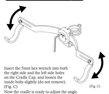
After adjustment, tighten both bolts firmly to fix the position.
