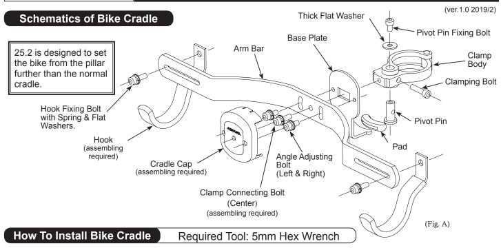
The clamp body has been pre-installed on the pillar. You will install the bike cradle to the clamp. The hook and the cradle cap are separated. You will install them on the cradle later.
