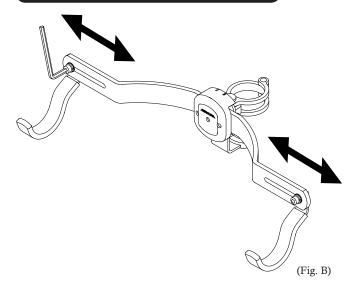
Take the bike off the cradle. Loosen the bolt and slide the hook to adjust the position. You should set the hooks symmetrically to maintain maximum bike stability.
