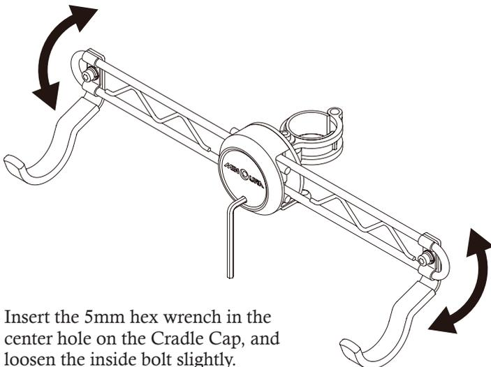
Insert the 5mm hex wrench in the center hole on the Cradle Cap, and loosen the inside bolt slightly. Then insert the hex wrench into the lower hole, and loosen the inside bolt. Now the cradle is ready for adjusting its angle. After adjustment, tighten both bolts firmly.
