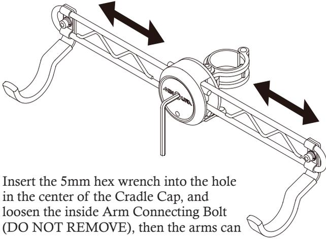
Insert the 5mm hex wrench into the hole in the center of the Cradle Cap, and loosen the inside Arm Connecting Bolt (DO NOT REMOVE), then the arms can move.
