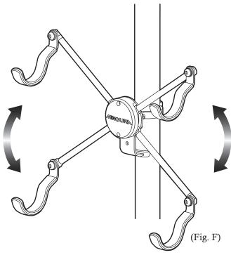
Each arm is angle adjustable in +/- 35 degrees in order to fit various types of bike frames as perfectly as possible (see Fig. F).
