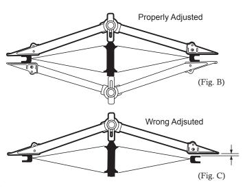
Set the wheel on the wheel truing stand to adjust. To know how to adjust the wheel, refer the instructions manual of the wheel truing stand.
