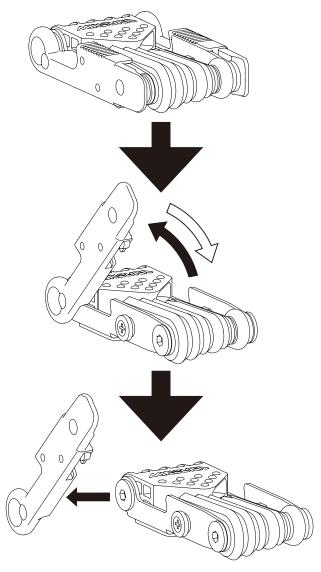
To remove the tire lever, simply turn upward then pull out.
