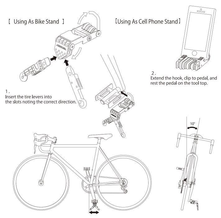
3. Set crank arm back slightly so the bike leans at 10 degrees.
