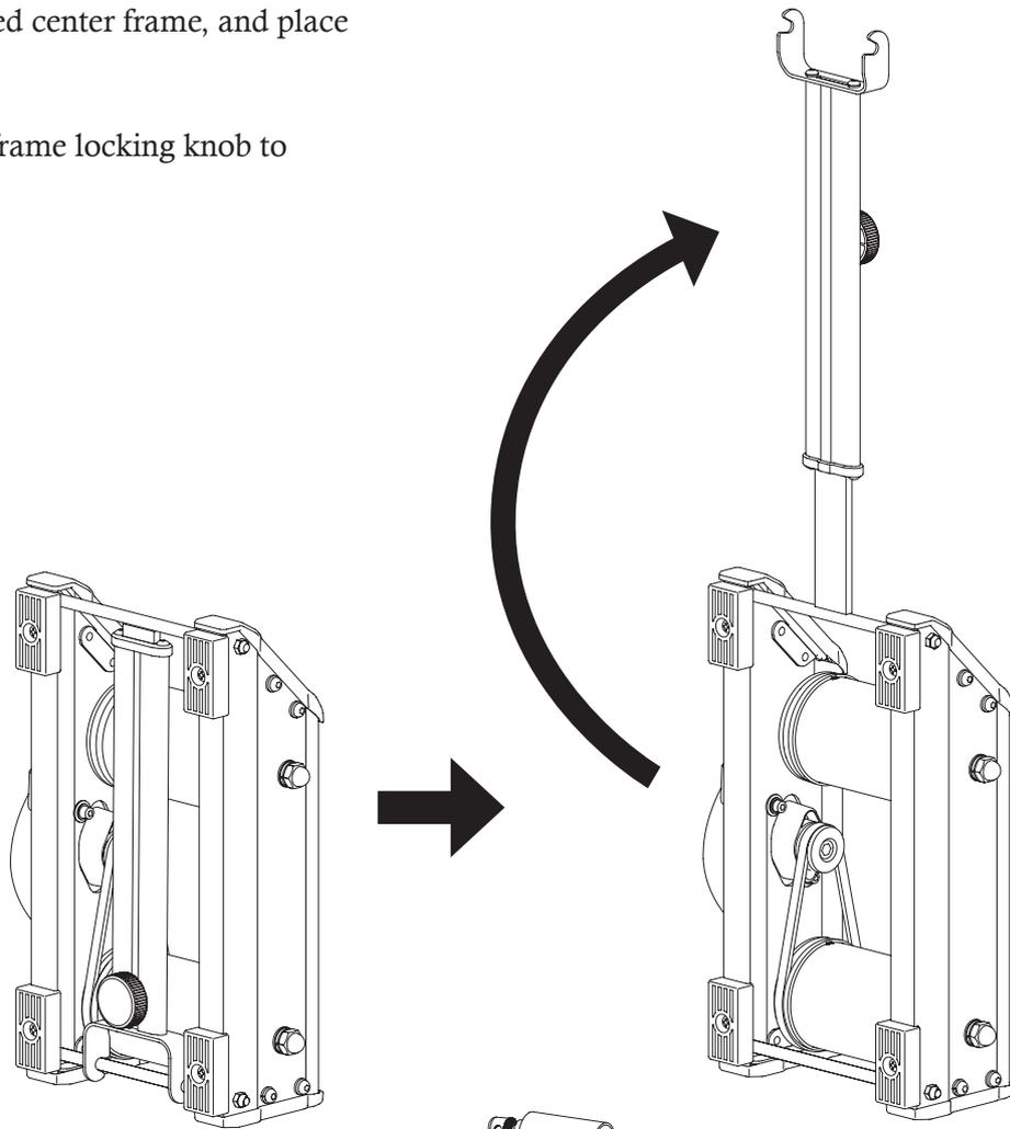
**3** Connect the center frame to the tripod center leg. Tighten the Q/R firmly.
