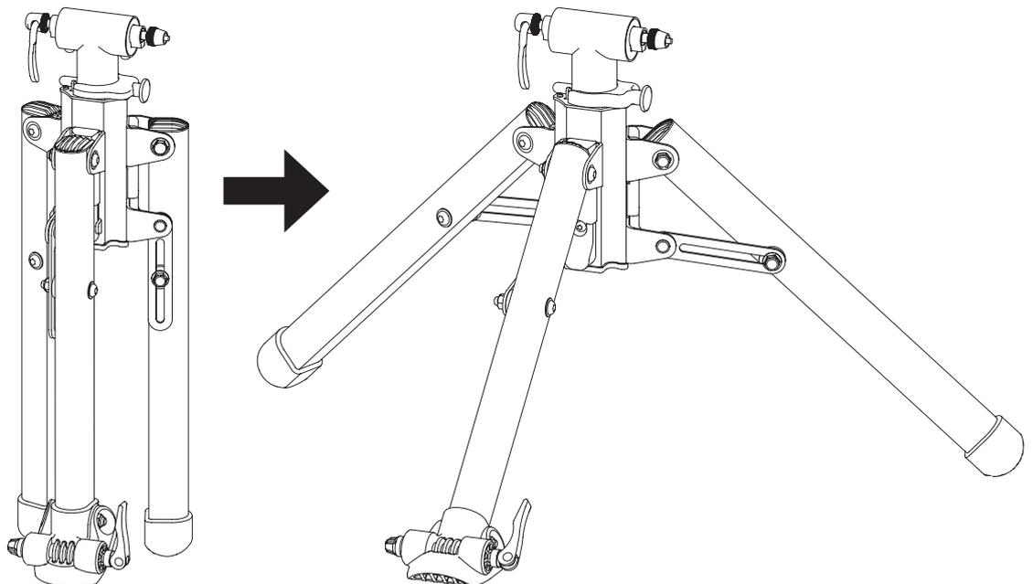
**2** Flip out the retracted center frame, and place on the floor.
