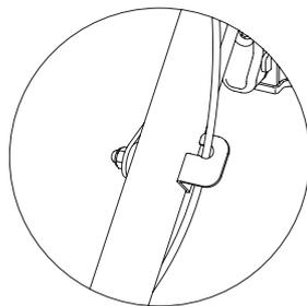
There is a guide bracket on the right side tripod leg to hold the remote cable.
