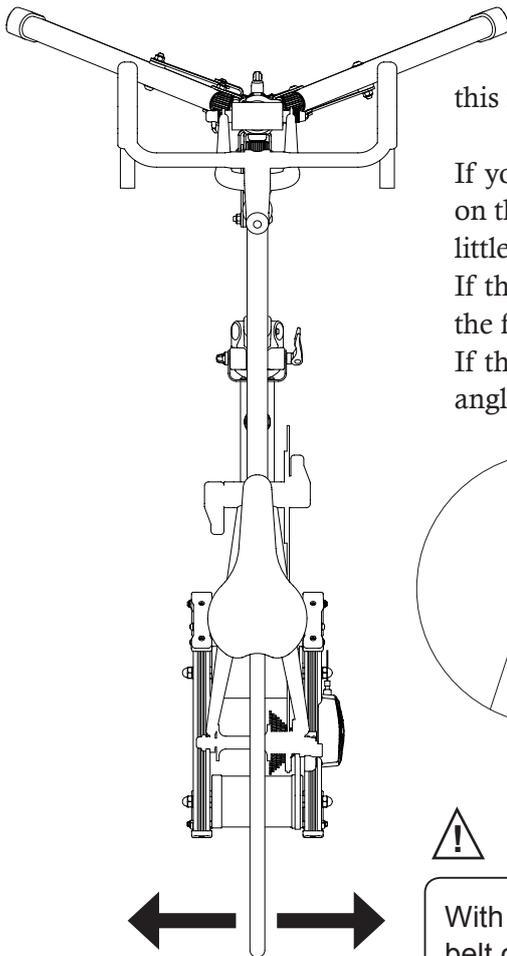
It's normal for the rear tire to sway or move back and forth slightly while using. As long as the tire doesn't touch the sides of the rollers this is ok.
