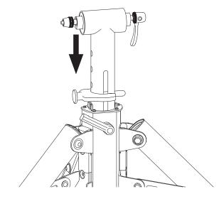
The stopper pin can be removed only while the fork mount is lifted up.
