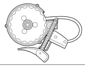
Pull out the Pulley Arm from the Mag unit.
