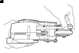
Now the Main Arm can be removed to replace the V-Belt.
