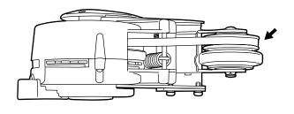
There are two types of Pulley Arm. The older one has just one hole, and the latest one has two holes. Use the upper hole in the beginning, then switch to the
