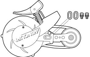
6 Remove 3 screws from the outer edge and 2 screws
