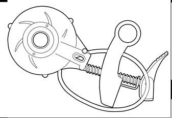
Turn the pulley to fit the belt.
