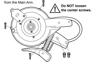
Push the Pulley Arm to come off the V-Belt.
