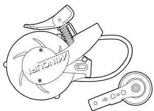
Loosen the Nylon nut to remove the Alloy Rotor.
