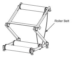
Fold the frame to loosen the roller belt tension.
