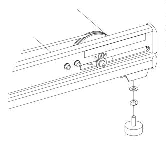
There are 6 Foot Adjusters in total under the R800 side frames. Each one is installed on each bottom bracket. Adjust the foot height inidividually as all 3 roller drums become completely horizontal and parallel when all 6 foot points touch the floor.
