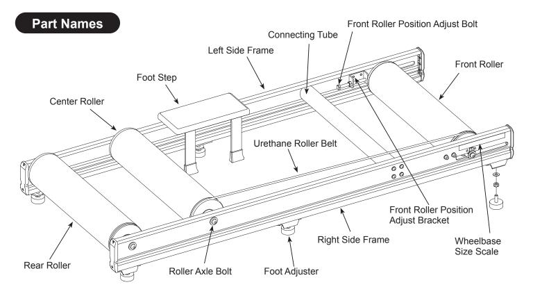
The Foot Step is fixed on the left side frame only because there is no hole on the right side frame. The roller belt is located on the opposite side to the step, so it is fixed on the right side only. It is not possible to change it to the left side by changing all roller drum directions.
