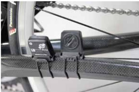
Attach the supplied **Speed magnet** on one of the spokes so that it lines up roughly with the **Speed sensor** on the chain stay. Ensure that the flat surface of the speed magnet is facing the Speed sensor and that the 'slot' side of the speed magnet is facing the hub.
