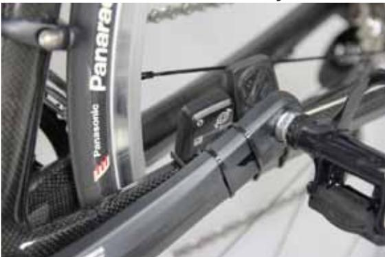
Usually there is a depression on the inside of the crank arm that this will sit in quite nicely. When you turn the crank arm, the (middle of) **Cadence magnet** should line up with the 'S' on the upper left corner of the **Cadence sensor**.
