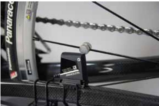
When you turn the crank arm, the (middle of) Speed magnet should line up with the 'ALLOW' on the upper left corner of the **SPEED sensor**.
