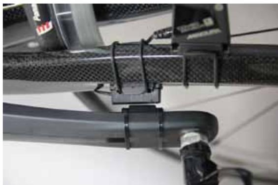
Tilt the **Cadence sensor**. out toward the crank arm so that it is roughly 2-5 mm away from the **Cadence magnet** (or as close as you can without them touching) on the crank arm when you turn the pedal.
