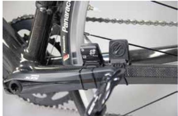
Attach the **Cadence magnet** 'loosely' onto the inside of the crank arm using the zip ties toward the pedal end so that it lines up roughly with the **Cadence sensor** on the chain stay.
